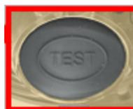
As an important item of safety equipment, your EPIRB should be checked regularly. The EPIRB has a built-in test capability that can be used as a confidence check. This self-test confirms that the battery is healthy, that the GPS receiver and both distress
